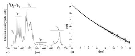
Fig. 4. (a) Luminescence emission spectra of YSO:Eu<sup>3+</sup> sample excited at 393 nm. (b)  $^5D_0$  decay profile at room temperature (the decay times  $\tau_1 = 1.451$  ms and  $\tau_2 = 2.893$  ms).
