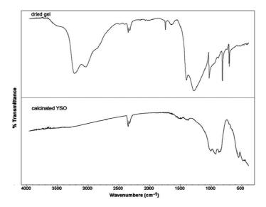
Fig. 2. FTIR spectra of dried gel and calcinated YSO:Eu<sup>3+</sup> sample.
